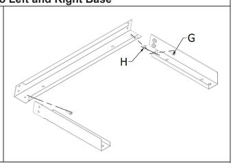
Attach Front Base (A) to the Left Base (D) and Right Base (E) and secure them with 2 of the M6\*12mm Screws (G) and 2 of the M6 Flange Nuts (H) using a Phillips Screwdriver (not included).
