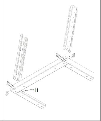
Attach Left Vertical Rail (B) and Right Vertical Rail (C) to the frame built above and secure them with 8 of the M6\*12mm Screws (G) and 8 of the M6 Flange Nuts (H) using a Phillips Screwdriver (not included).
