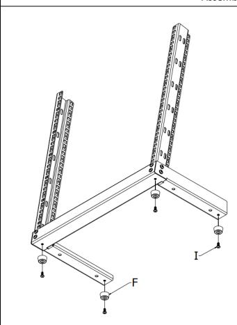
Attach 4 Plastic feet (F) to the frame built above and secure them with 4 of the M5\*12mm Screws (I) using a Phillips Screwdriver (not included).
