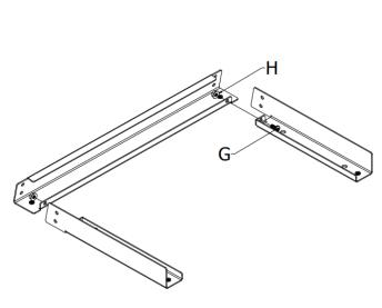
Attach Front Base (A) to the Left Base (D) and Right Base (E) and secure them with 2 of the M6\*12mm Screws (G) and 2 of the M6 Flange Nuts (H) using a Phillips Screwdriver (not included).
