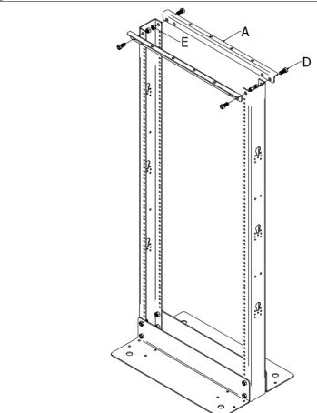
Connect Top Brackets (A) to the combined Vertical Rack Rails with 8 of the 3/8"-16 Hex Bolts (D) and 8 of the 3/8"-16 Nuts (E) using Wrench (H).
