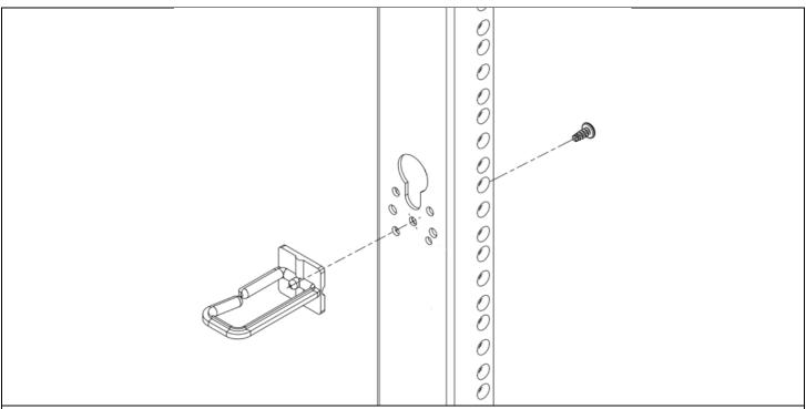
Optional: Fasten the included Cable Management Hooks (G) to the vertical rack rails with the included Hook Mounting screws (F) using a Phillips Screw Driver (not included).
