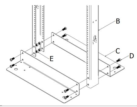
Connect Vertical Rack Rails (B) to the Base Brackets (C) with 8 of the 3/8"-16 Hex Bolts (D) and 8 of the 3/8"-16 Nuts (E) using Wrench (H).
