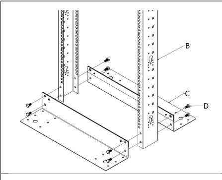
Connect Vertical Rack Rails (B) to the Base Brackets (C) with 8 of the M8 x 16mm Hex Bolts (D) using M8 Wrench (J).
