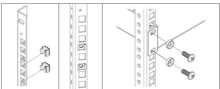
1 Locate the numbered square openings in the mounting rails where you plan to install your equipment. You will install cage nuts (included) into the square openings in order to provide an attachment point for the mounting screws (included). Note: Consult your equipment documentation to determine how many cage nuts will be required and where they will need to be installed.
