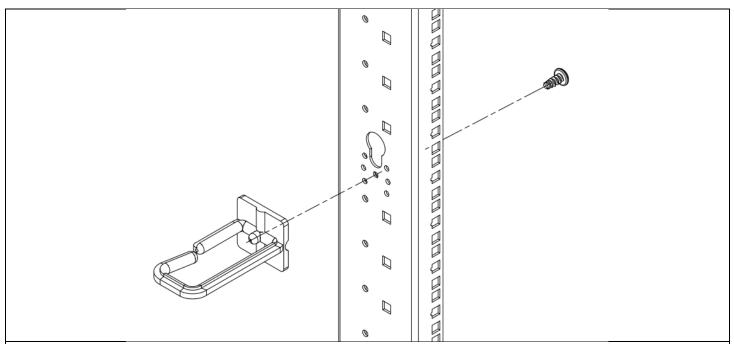
Optional: Fasten the included cable management hooks (I) to the vertical rack rails with the included screws (H) using a Phillips Screw Driver (not included).
