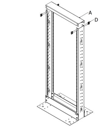
Connect Top Brackets (A) to the combined Vertical Rack Rails with 8 of the M8 x 16mm Hex Bolts (D) using M8 Wrench (J).
