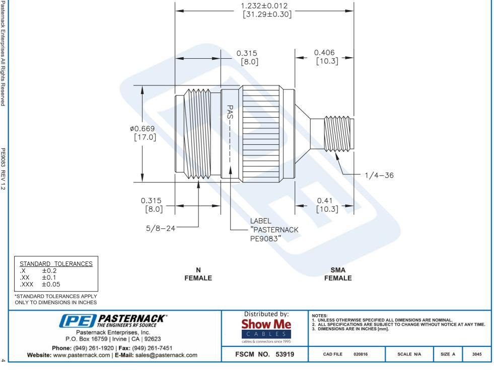
PE9083 CAD Drawing SMA Female to N Female Adapter With Knurl
