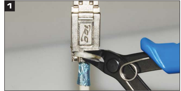
Step 1. 1.) Cut the cable tie. NOTE: Do not cut or damage the drain wire.
