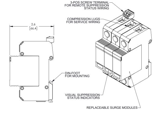
UNLESS OTHERWISE SPECIFIED LEADING DIMENSIONS ARE INCHES DIMENSIONS IN [] ARE MILLIMETERS
